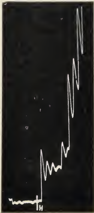
FIG. 224. Effect of application of warm water II in increasing sap-pressure in a shoot in the condition of balanced turgor.
